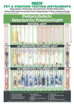
Preform Defect Chart is a consistent tool useful for visual assessment and evaluation of defects found in PET preforms. Used in various industries and laboratories to maintain quality and consistency of a sample to detect the defects under natural and polarized lights. Available with Polariscopic Deluxe Model also.
